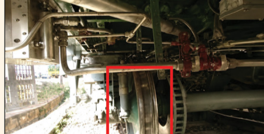
Missing Bolt/Axel Box Detected
