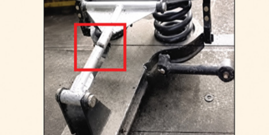
Axel Cap Missing & Bogie Frame Crack Detected
